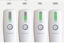
Check the charge status on the light bar:
