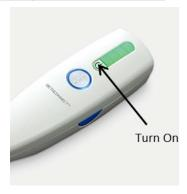
Before turning BETACONNECT on, make sure BETACONNECT is within operating temperature. If stored below 41°F (5°C), wait at least 4 hours before turning BETACONNECT on.
